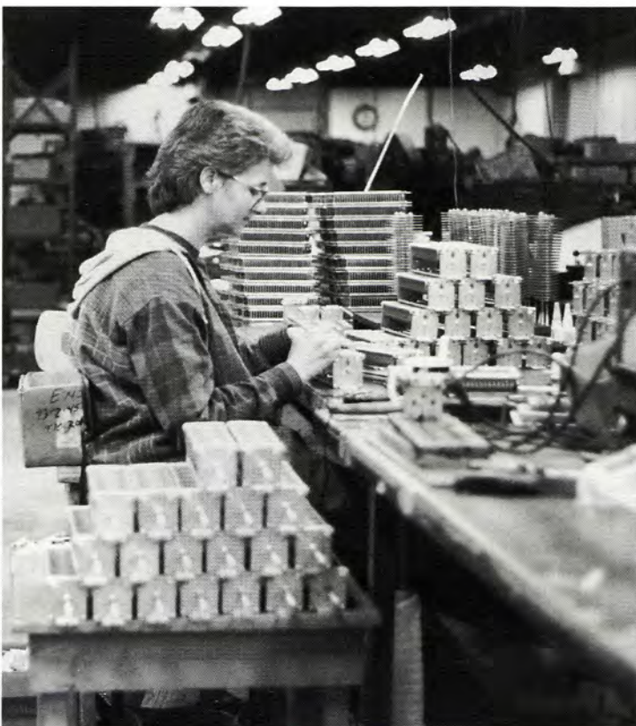
Before shipment, every M-73 undergoes maximum voltage testing.
