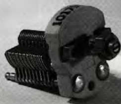
APC75G with type C shaft and lock bearing, #1 spider position, and 3/32" mounting posts
